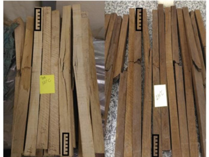
**Figure 3.** Image of the specimens after the mechanical testing, highlighted by the black ruler icons where the material was removed for the physical tests.
