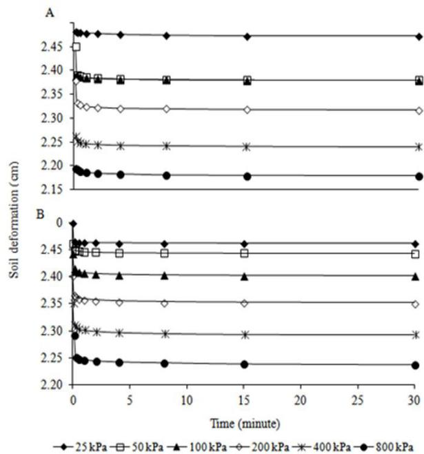
Figure 1. Soil deformation versus time of load application to conventional management (A) and no-tillage (B).
