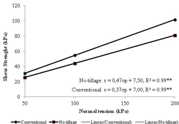
**Figure 4.** Shear strength ( $\tau$ ) versus normal tension ( $\sigma_p$ ) of the soil in the conventional tillage and no-tillage.
